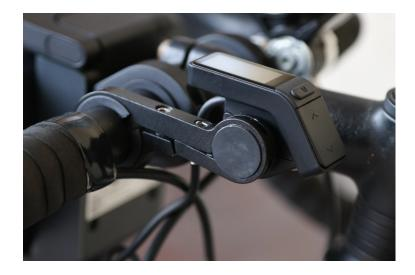
The display is neat, and designed for flat handlebars, which means you won't be able to fit it directly to a drop bar, as the diameter of the mount is too small. I've used half of a bar extension thing I got from Temu, and that works really well. Then it's just a case of joining up all the wires, zip-tieing them in place, and charging up the battery ready to go.
