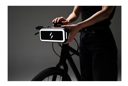
The Swytch conversion kit can upgrade almost any bike into a legal pedal-assist electric bike with a top speed of up to 15 mph and a power output of 250W. It works by replacing your regular bike wheel with a custom-built Swytch motor wheel (made locally at Swytch's factory in Norwich, UK), which is connected to a battery that can be easily removed and mounted on the handlebars, delivering 250W of pedal-assist power when you start pedaling.
