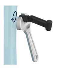
2.1 The peg should bend downwards and line up with the latch on the Brompton forks. This might take a few adjustments to align perfectly.
