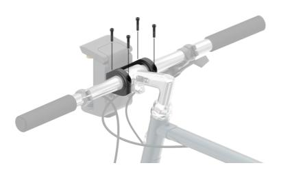
1.2 To lower your bracket, first use the 3mm Allen key to remove the the two M5 bolts and lower half of the bracket piece.
