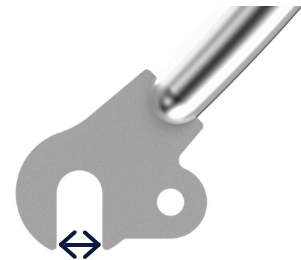
10mm or 9mm fork dropout
