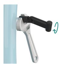
2.1 The peg should bend downwards and line up with the latch on the Brompton forks. This might take a few adjustments to align perfectly.
